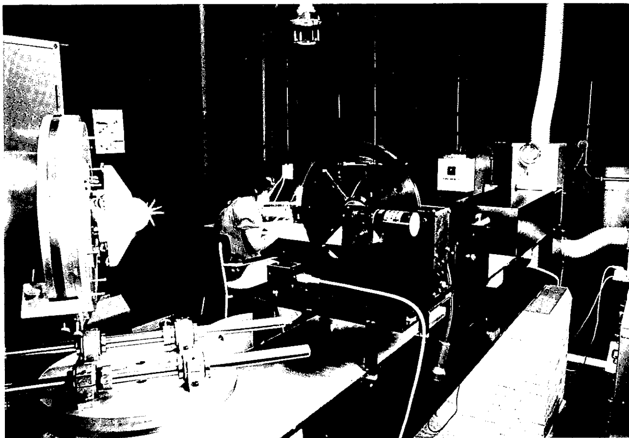
Figure 1a. Photo of Kipp & Zonen sun simulator
